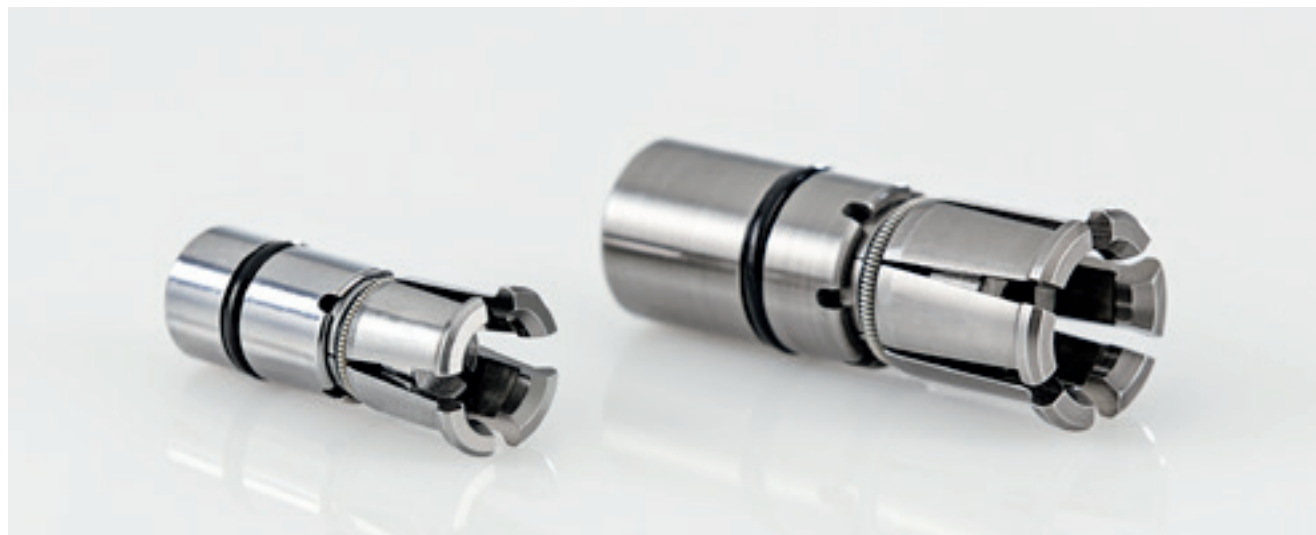
Grippers for tool holders ISO 10 and ISO 20 with guided segments for high-speed machining spindles and with short clamping strokes enabling long-lived spring stacks (type SSKFI ... ISO) ↑
